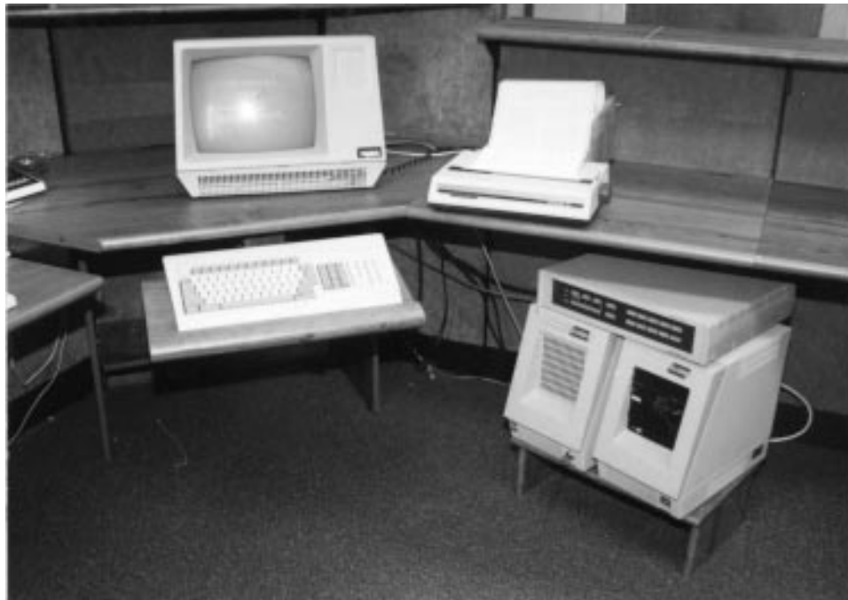
Figure 3-6.—Real-Time Automated Personnel Identification System (RAPIDS) computer used to access DEERS by personnel at PERSUPPDETs.
